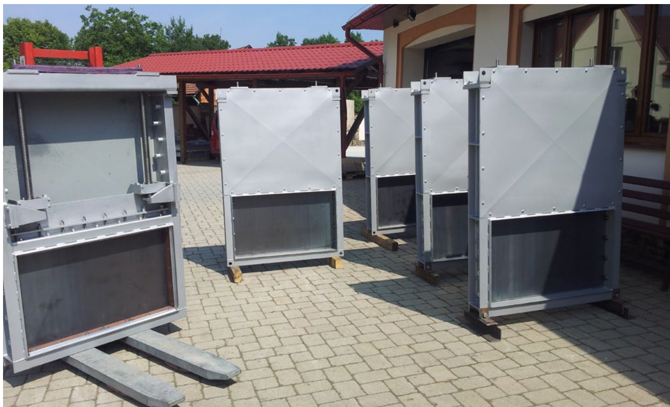
Production of blanking plates and butterfly dampers for Denox
