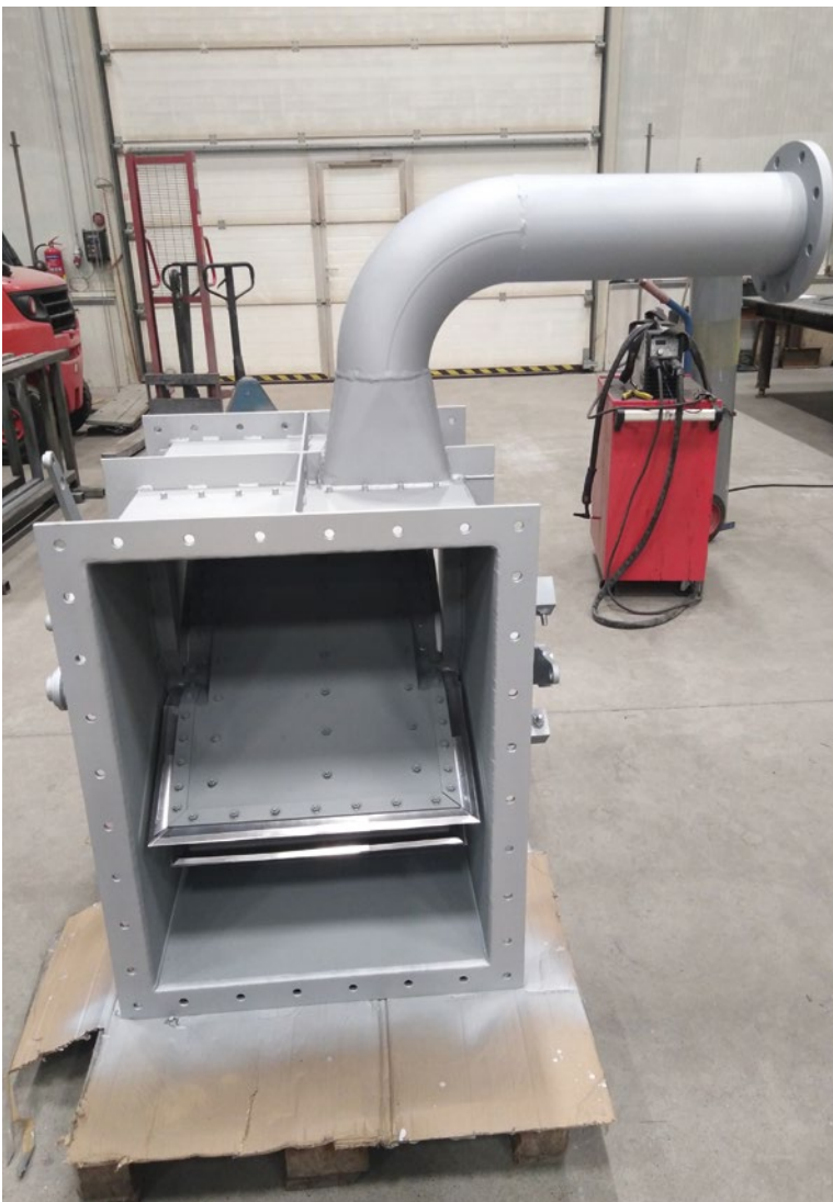
Production of 100% airtight damper with sealing air
