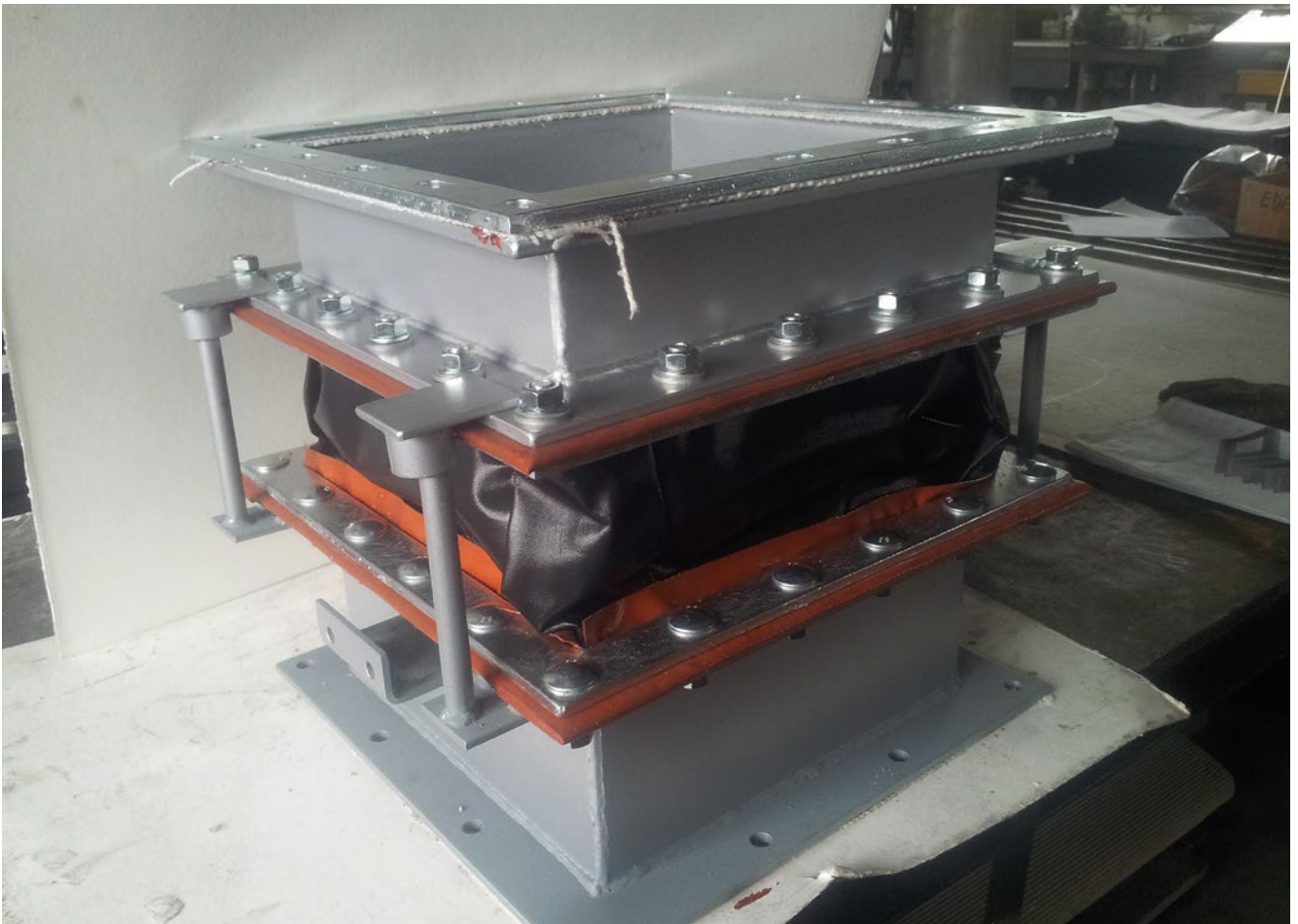
Production and installation of a fabric belt expansion joint instead of a flange type, including steel components
