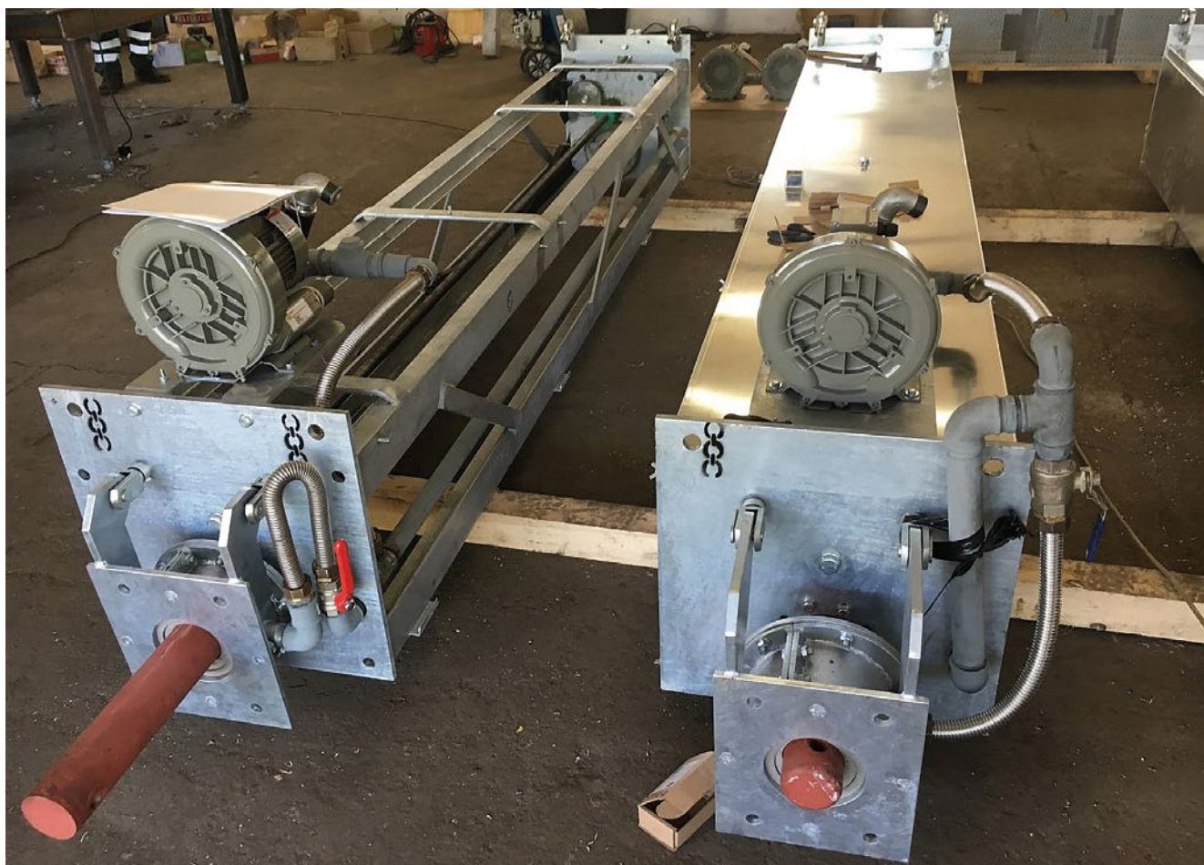
Supply of fully retractable soot blowers
